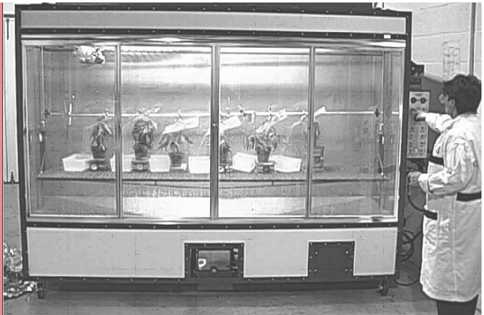
A rainfall simulation chamber was used to measure the ability of eight insecticides to uphold under various precipitation patterns.
